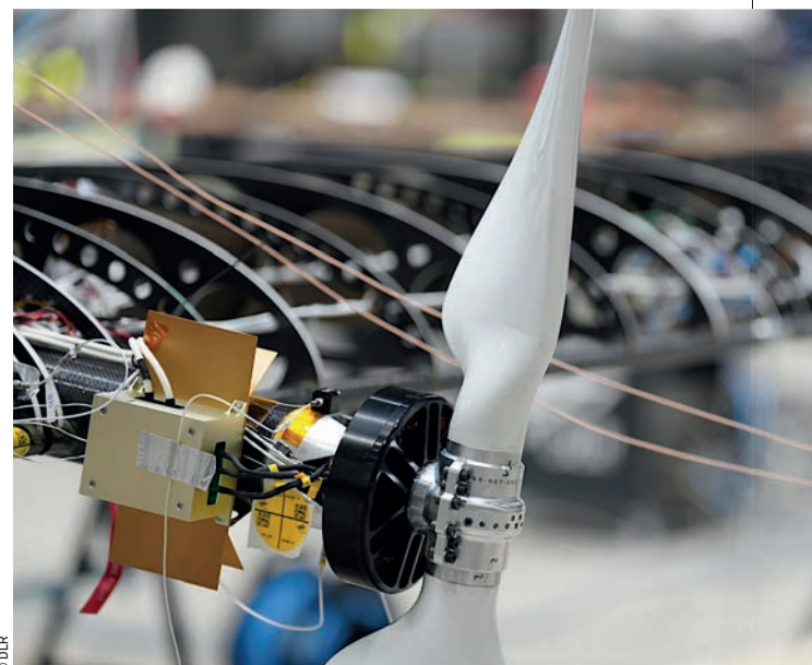
Electric motor on the wing of HAP-alpha, equipped with acceleration sensors
