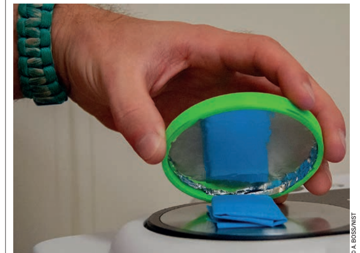
A clothing sample is analyzed using an analytical lab technique called near-infrared spectroscopy. The method measures how much of the light passes through or scatters off the fabric, producing a unique pattern — a sort of fingerprint that can identify the types of fibers in clothing
