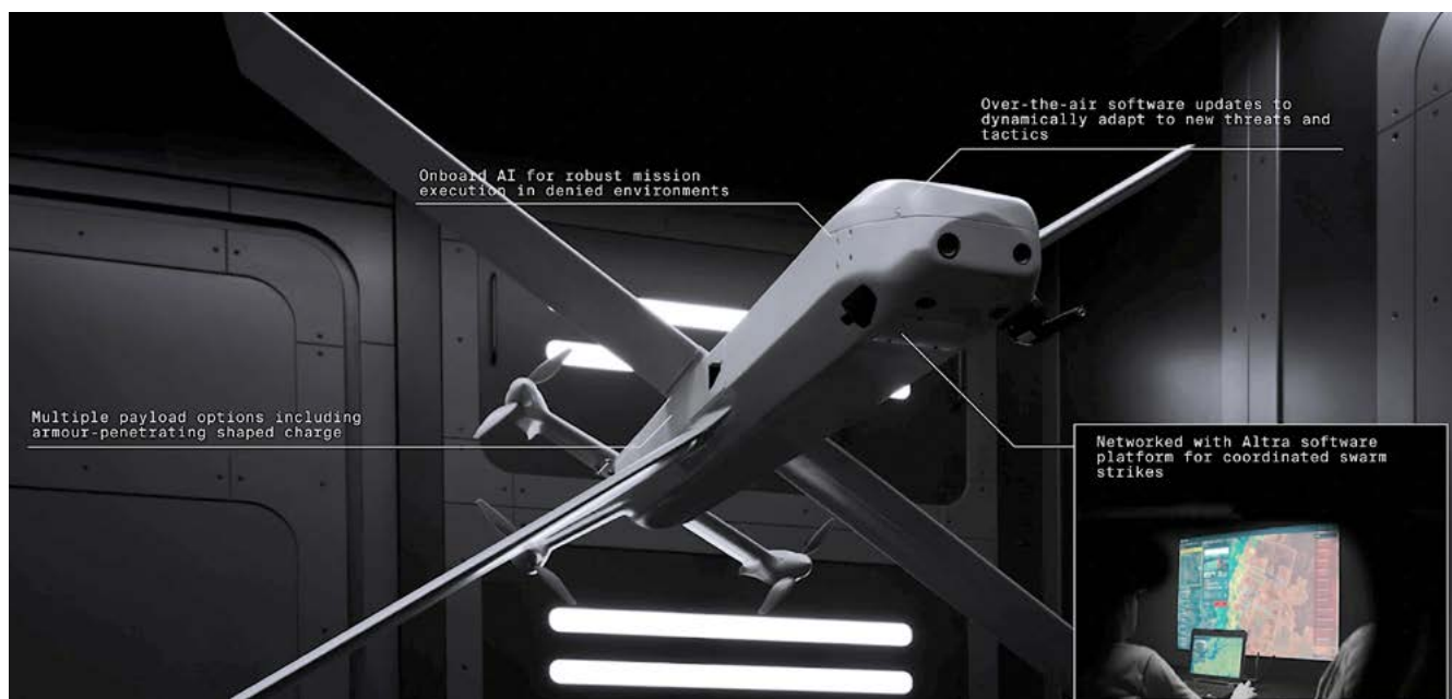
Helsing's HX-2 is a new type of strike drone capable of engaging artillery, armoured and other military targets at beyond-line-of-sight range (up to 100km)
