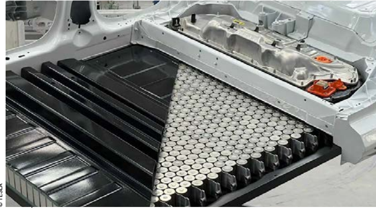
An LFP battery such as this Tesla battery is a lithium iron phosphate battery that uses iron phosphate as the cathode material
