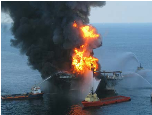
The Deepwater Horizon was an ultra-deepwater, dynamically positioned, semi-submersible offshore drilling rig that sank on April 22, 2010, after an explosion and fire, killing 11 crew members
