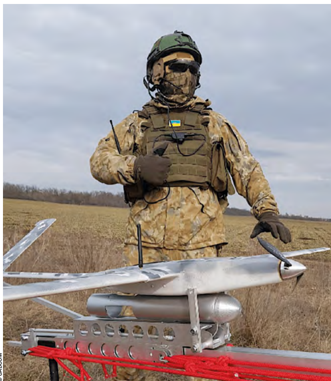
The SKYFIST drone manufactured by the Ukrainian company Uadcom can be armed with 75mm explosive bombs
