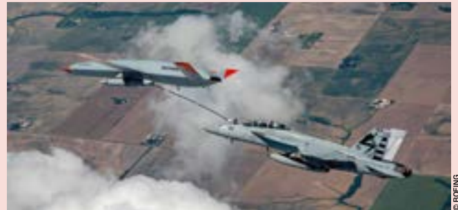
A test version of the MQ-25 has successfully refuelled the F/A-18, F-35C and Northrop Grumman E-2D Hawkeye.
