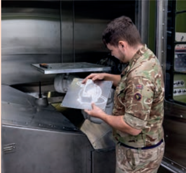
A Sapper from the Royal Engineers removing a part from the cold metal 3D printer
