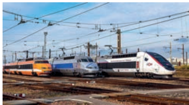
The three TGVs having held the world rail speed record, lined up at Villeneuve Saint-Georges (France), for the 40th anniversary of the launch of the TGV services . •TGV Sud-Est n° 16 (380 km/h in 1981) • TGV Atlantique n° 325 (515,3 km/h in 1990) ;• TGV POS n° 4402 (574,8 km/h in 2007).
