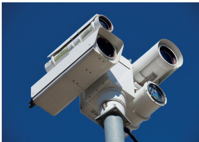
The cameras, night vision, and radar system of a Remote Video Surveillance System
