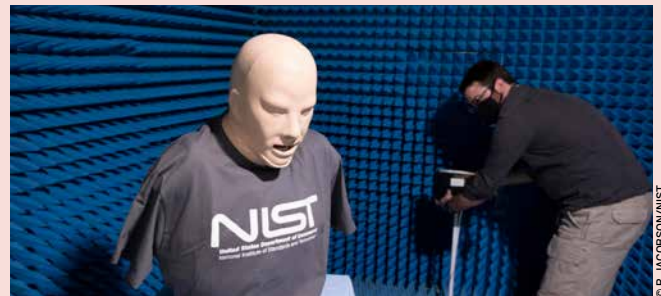
Jason Coder sets up an experiment in an anechoic chamber to use Wi-Fi to sense breathing. The manikin is used to train medical professionals, and simulates a number of breathing scenarios
