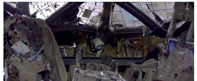
The airplane was perforated by hundreds of high energy objects shaped like cubes and bow-ties. Many preformed fragments were in the bodies of the crew seated in the cockpit
