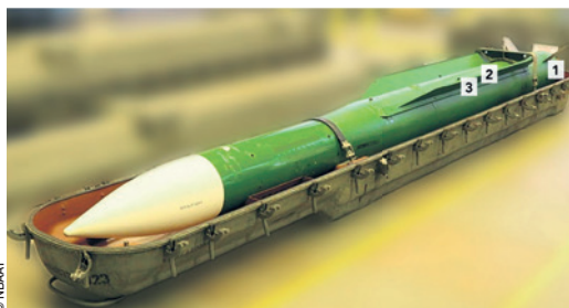
Image of 9M38M1 surface-to-air missile showing the approximate location of three of the parts recovered
