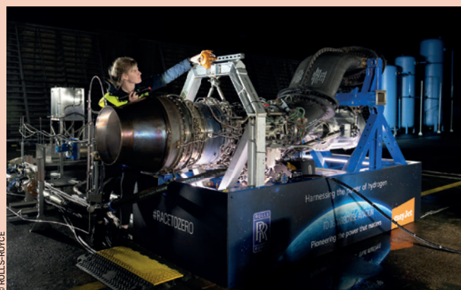
Rolls-Royce AE2100 Hydrogen Test at Boscombe Down, UK
