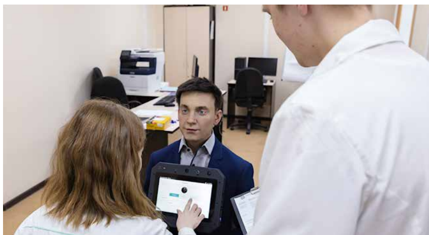
The "face" of Robo-C can display more than 600 variants of human facial expressions: the robot can move its eyes, eyebrows, lips, neck and "face muscles"
