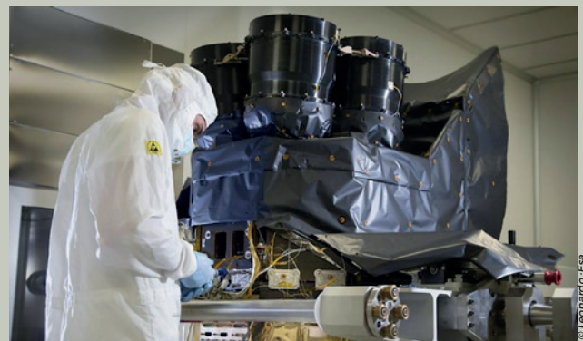
Meteosat Third Generation Imager-1's Lightning Imager during testing at Leonardo's facilities in Florence, Italy. The Lightning Imager will provide a new capability for European meteorological satellites. It provides a continuous monitoring of more than 80% of the Earth disc for detecting lightning discharges taking place either between clouds or from cloud and ground
