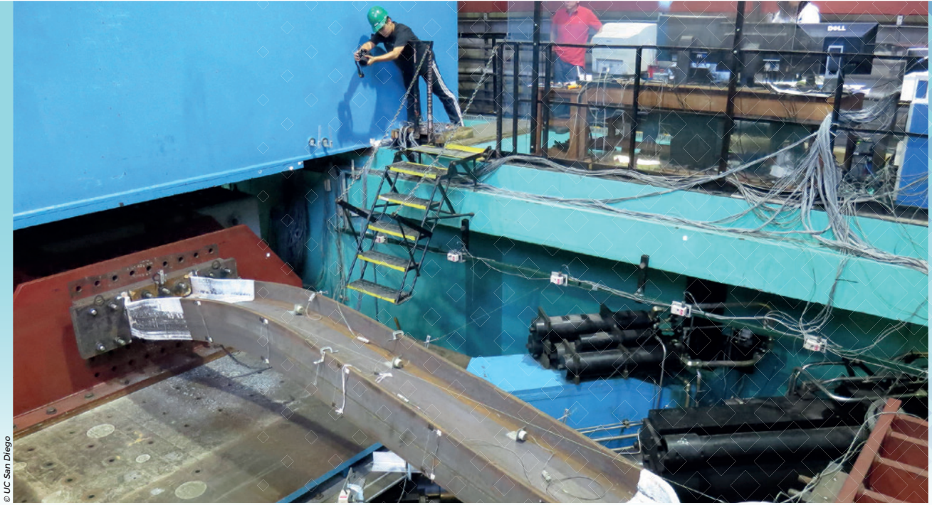
The researchers fastened 48 steel columns of varying dimensions into a hydraulic system called a shake table that thrusts one end of each column back and forth, replicating the shaking motions of an earthquake
