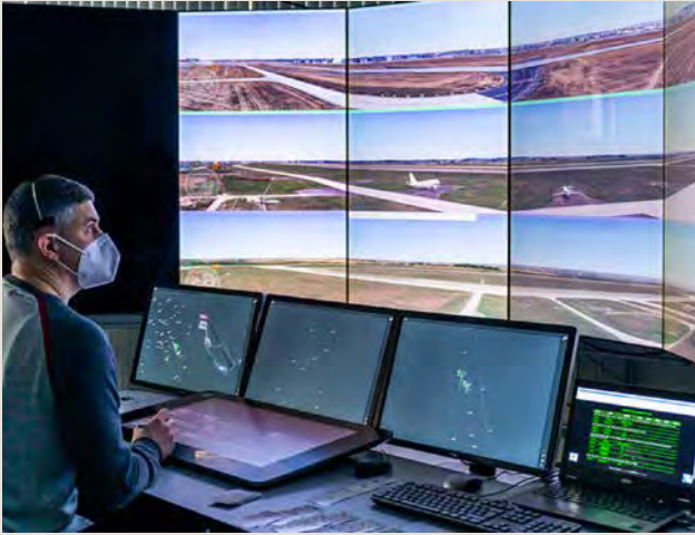
An air traffic controller is simultaneously responsible for three remote airports supported by outside views, radar displays, and visualization of speech recognition outputs in an electronic flight strip display
