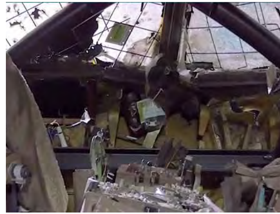
The airplane was perforated by hundreds of high energy objects shaped like cubes and bow-ties. Many preformed fragments were found in the bodies of the crew seated in the cockpit
