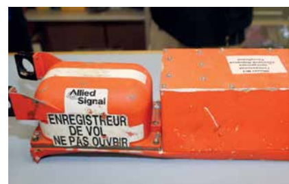
Flight data recorder without Underwater Locator Beacon. Source Dutch Safety Board. Cockpit Voice Recorder
