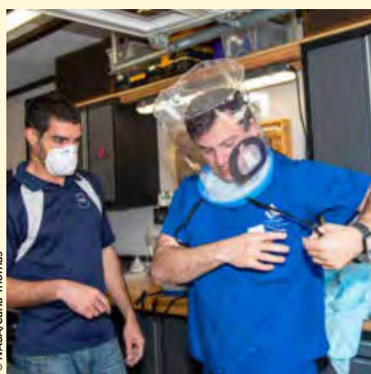
NASA engineer Mike Buttigieg works on an oxygen hood system prototype worn by Dr. Daniel Khodabakhsh from the Antelope Valley Hospital in California. The hood is designed to help coronavirus patients who don't yet need a ventilator, but who are experiencing breathing troubles. The hood forces oxygen into patients with mild coronavirus symptoms, minimizing the likelihood that the patient will need to use a ventilator
