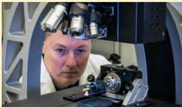
Thomas Brian Renegar examines the positioning of the bullet before the scanning run begins. Twenty-two such scanning runs were needed to fully capture all the surface details of the stretcher bullet from every angle, resulting in 1,699 individual measurements of the bullet’s surface.
