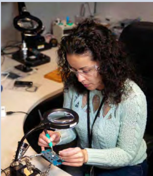
NIST computer scientist Jenise Reyes-Rodriguez uses the JTAG method to acquire data from a damaged mobile phone.
