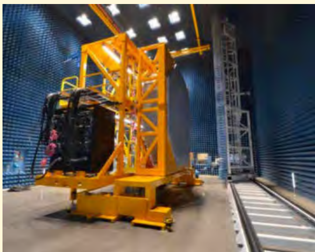
The U.S. Navy's SPY-6 integrated air & missile defense radar in production at the Raytheon Technologies Radar Development Facility in Andover, Massachusetts.
