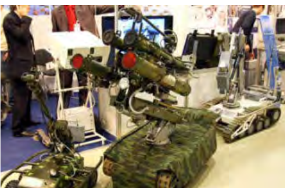
MRK-27 BT with RShG-2 and RPO Shmel is a vehicle intended for bomb disposal equipped with a 7.62mm machine gun, RShG-2 rocket-propelled assault grenades and the thermobaric weapon RPO-A SHMEL
