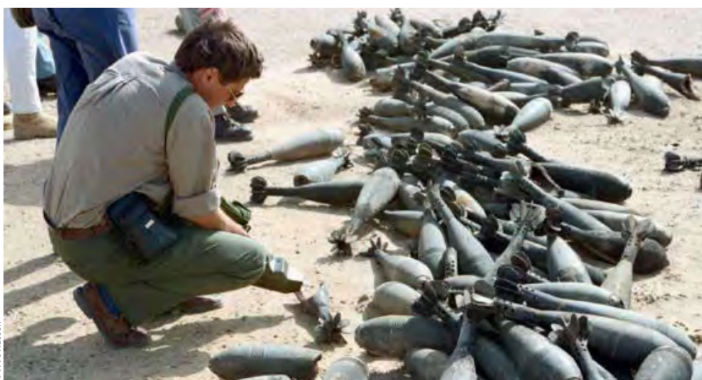
A member of the UN Special Commission (UNSCOM) inspection team uses a chemical air monitor to detect leakage from a CS-filled 120mm mortar shell at Fallujah Chemical Proving Ground, as part of the inspection to verify Iraq's compliance with the order to destroy the chemical munitions for chemical weapons and weapons of mass destructions in 1992
