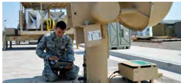
A Squadron ground control station maintainer, powers a ground data terminal used to transmit signals needed to fly both the MQ-1B Predator and MQ-9 Reaper
