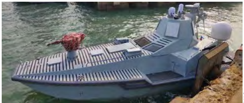
China's new killer robot ship JARI, is designed for remote-control or autonomous operation
